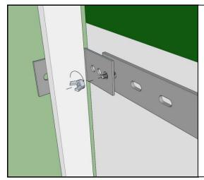
Bring the brackets together and line up the bolts with the holes on the small brackets. Choose the holes that best secure your Waterboy Unit in place. Then attach and tighten the provided wingnuts to the bolts.
