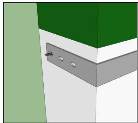
Place the large bracket on the front of your Waterboy Unit at an appropriate height to keep it secure. Ensure the provided bolts are in position on both sides.
